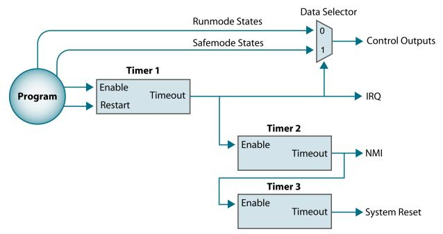
As in the previous example, a Timer1 timeout will switch the outputs to safe states, start Timer2, and request interrupt service. If the computer is able to respond to the IRQ, the program will attempt to recover from the fault condition and, if successful, the program will disable Timer1 (and by extension, Timer2), thus canceling further corrective actions.
