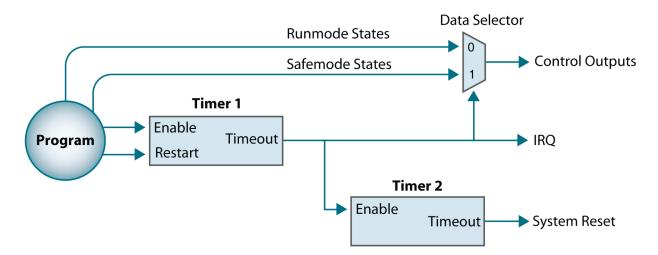
During normal operation, the program kicks Timer1 at regular intervals to prevent it from timing out. As long as Timer1 has not timed out, Timer2 is disabled and held at its initial value, and the control outputs are allowed to change under program control.
