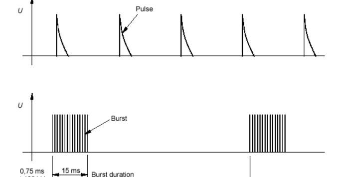
Figure: EFT/Burst Waveform
