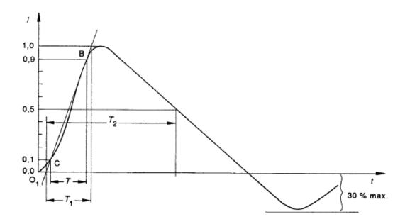
Front time:  $T_1 = 1.25 \times T = 8 \mu s \pm 20 \%$
