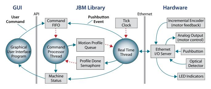
As shown in the above diagram, the JBM library has two threads. The command processor thread is responsible for managing overall machine state. The command processor thread receives and executes commands from the GUI and pushbutton, and it computes and issues the motion profiles needed to satisfy those commands.
