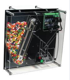
the bucket will deliver the jellybeans to the exit chute. The reservoir is assumed to be empty if the bucket comes up empty on a second pass.
