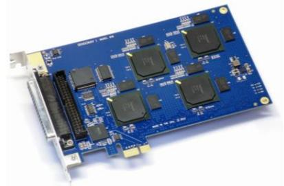
An internal 16 X 4 analog crosspoint video switch is used to route any combination of four composite output channels to external video monitors. Individual scalers and deinterlacers facilitate optimal resolutions for each captured stream. For example, a high-resolution, high bitrate stream may be selected for archiving, while a lower resolution, low bitrate stream is preferable for simultaneous streaming to handheld devices, including smart phones.
