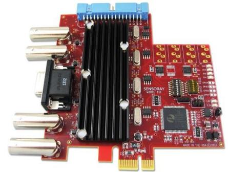
Four BNC connectors are available on the board's mounting bracket for connecting external composite video sources. A DB15 connector on the same bracket is used for the audio inputs. A 34-pin header provides an alternative convenient access to all I/O signals on the board.
