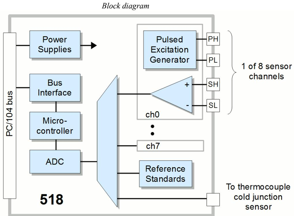
Pulsed excitation is provided for thermistors, resistors, RTDs, and strain gauges, which minimizes sensor self-heating and reduces power consumption. Excitation signals are routed to dedicated connector pins to allow four-wire sensor circuits that completely eliminate lead-loss errors.
