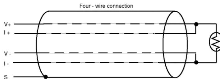
Thermistors have much higher resistance than RTDs over most of their operating range. As a result, a two-wire circuit may be used if your sensor will be operating only at higher resistance values. If it will be operating at lower resistance values, it is recommended to use a three- or four-wire circuit to prevent significant voltage losses.
