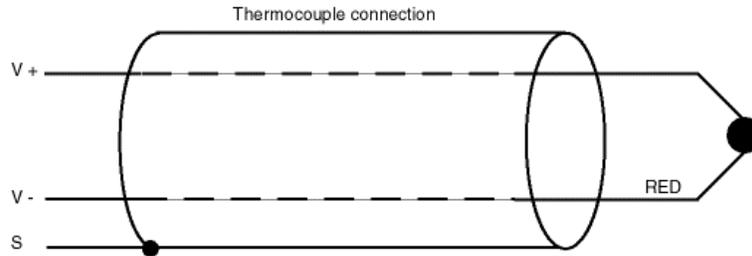
Electrical noise may be present on thermocouple and voltage signals. It is not within the scope of this manual to discuss all treatments of such noise, however, a few simple techniques are available which will solve many noise problems:
