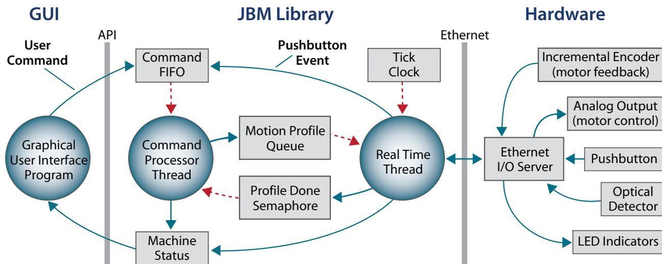
As shown in the above diagram, the JBM library has two threads. The command processor thread is responsible for managing overall machine state. The command processor thread receives and executes commands from the GUI and pushbutton, and it computes and issues the motion profiles needed to satisfy those commands.
